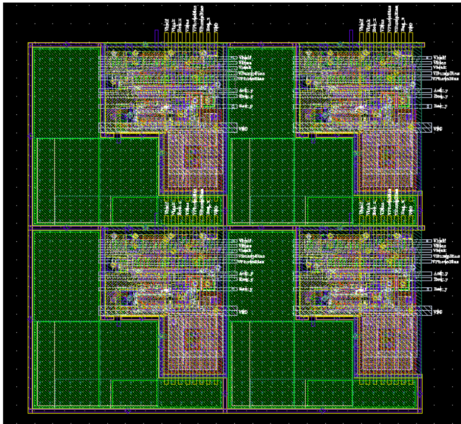
Figure D.3 Figure D.2 shows a 2x2 pixel-array with dynamic pixels.
