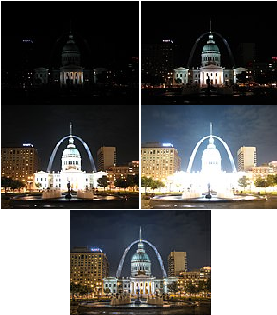
Figure 1.1: Four images of varying exposure (-4, -2, 2, 4) and the local tone mapping of the four images [7]
