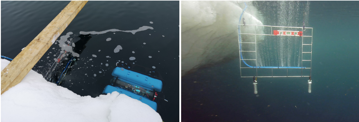
Figure 11: The ROV located in front of the bubble plane and the coordinate grid, which were lowered into the water by the pulley system, seen from above (left panel) and from the ROV perspective (right panel). A spirit level was used to align the coordinate grid with the horizontal.
