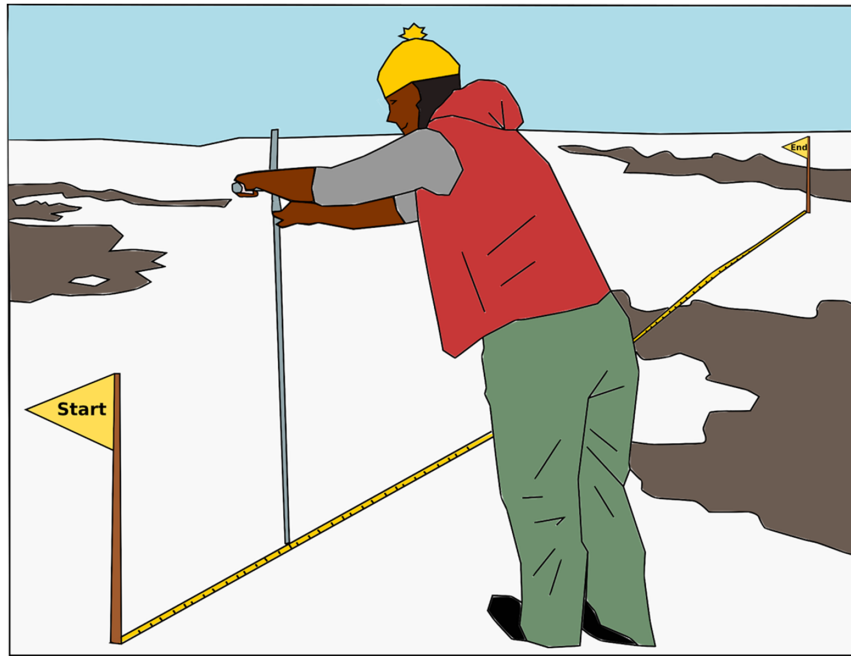
Fig. A3. Measuring snow depth on the transect during winter. This illustrates what a transect might look like.
