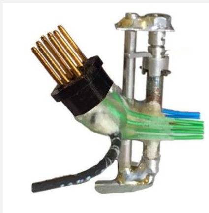
Figure 17 Base of microdrive recording device from Axona Ltd. The base is a re-usable drive with 16 channels with an additional fixed ground wire, attached to a steel frame and completed with a screw that makes it possible to move all tetrodes simultaneously. See: http://www.axona.com/products/microdrives .
