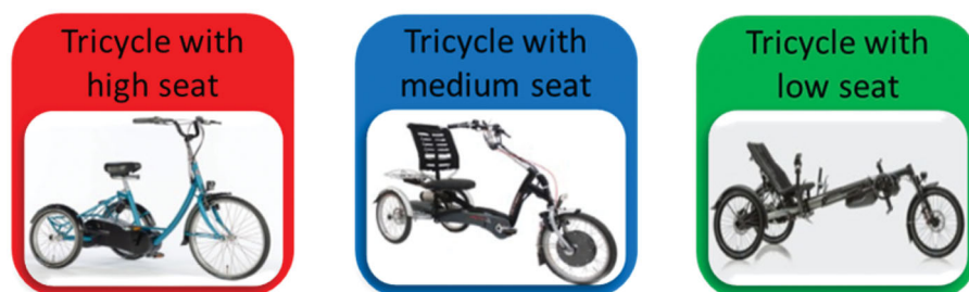
Figure 1. Images of the three tricycle categories. High seat = > 70 cm, medium seat = 57–63 cm and low seat = < 57 cm.
