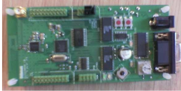
Figure 6.2: Chipcon CC2420DBK contains an 8-bit microcontroller that runs the implementation of the Device Control Protocol (DCP). The board supports the wireless IEEE 802.15.4 communication.
