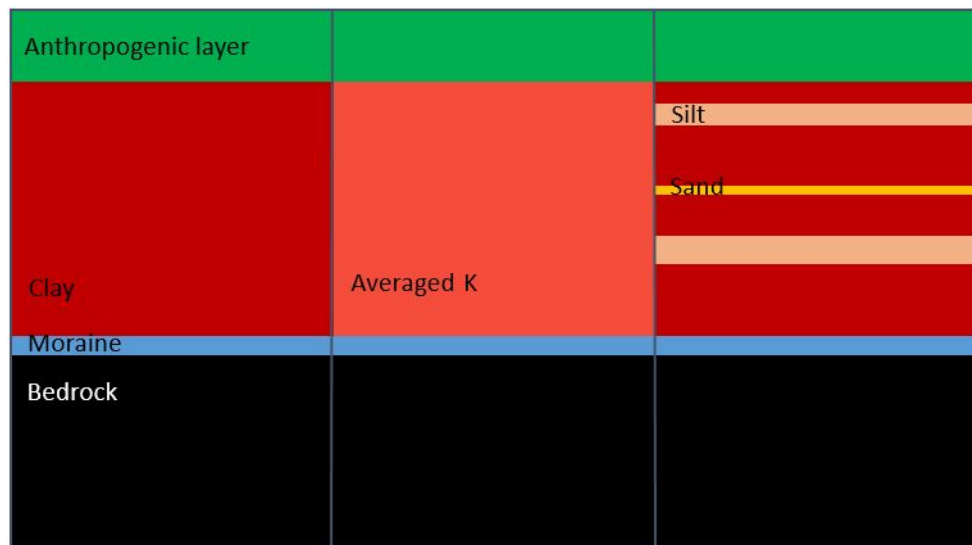
Figure 4.3: Three different stratigraphic scenarios will be applied for the sensitivity study. The layer thicknesses are not true to the actual relative sizes.
