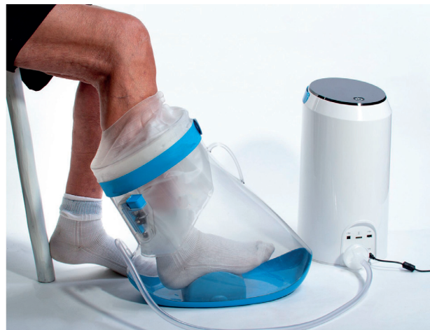
Fig 1. Device for lower extremity intermittent negative pressure treatment. Intermittent negative pressure is generated in a pressure chamber sealed around the patient's lower leg by a pump unit that is removing air from and venting the pressure chamber.
