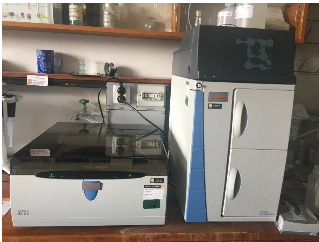
Figure D 2. Thermo Fisher Scientific Dionex Integrion HPICTM instrument.
