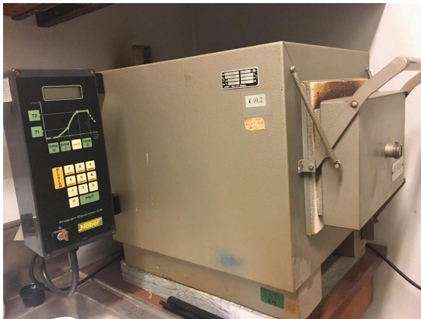
Figure C 1. Oven used for loss on ignition measurements of sediment samples.
