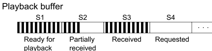
Figure 4.7: Snapshot of a stream in progress. The striped areas represent received data.
