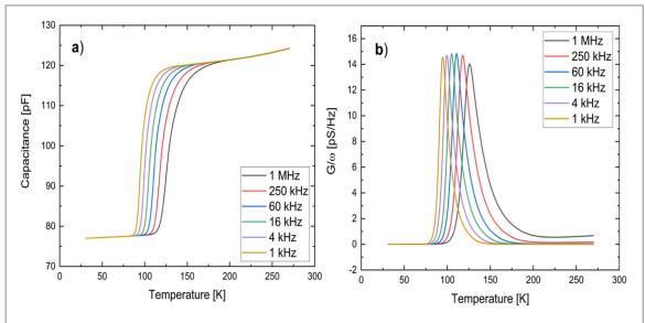
**Figure 4.** Capacitance (a) and conductance over angular frequency (b) simulated as functions of temperature for the 6 probing frequencies used in the experiment (1 kHz–1 MHz). The simulations are performed using the parameters in table 2.
