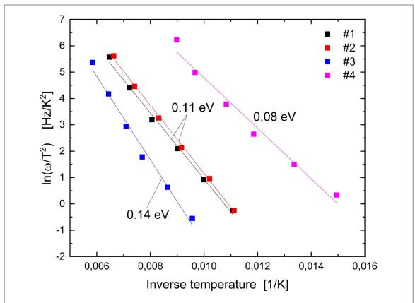
Figure 3. Arrhenius plot for TAS measurements of samples #1 - #4. The solid lines represent the linear fits. The deduced activation energies are indicated.
