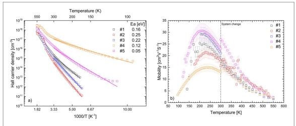
Figure 1. (a) Hole concentration versus inverse temperature in different samples. The solid lines indicate approximate fittings of the activation energies. The estimates of the activation energies are given in the parentheses. (b) Carrier mobility versus temperature in different samples.
