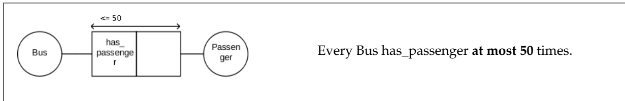
Figure 2.29: An ORM model with a frequency constraint.
