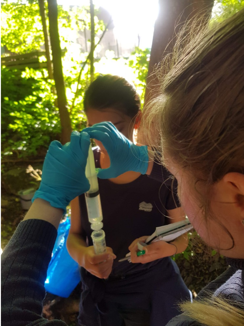
Figure A.9: Filtering of the water samples. Photo by Jorge Torres.
