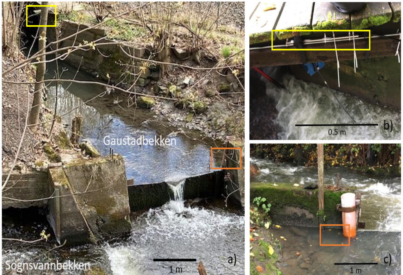
Figure 4.4: a) Picture of the Gaustadbekken weir after large disturbances were removed. The location of the logger is marked in a yellow rectangular and the location of the sensor is marked with an orange rectangular. The sensor is connected to the logger through a cable. b) Installed logger. Old equipment is visible under the logger as a blue box connected to a wire. c) Sensor installed in the river, marked by an orange rectangular. The sensor itself is not visible as it is under water.
