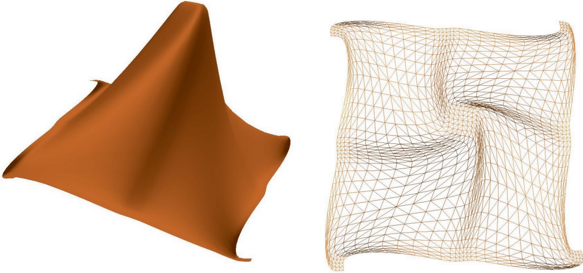
Figure 7.5: The “Tower” surface: a blending spline tensor-product surface made up by 3 \times 3 knots with an associated local plane surface patches. The local surfaces in the corners are locally rotated 90 degrees in the xy -plane and 45 degrees in xz -plane. The rendering lattice is here made up by 3 \times 3 render loci (one for each spline knot locus) and four render blocks. On the left is a shaded version of the resulting surface, while on the right is a wireframe version showing the tessellation of the four render blocks.
