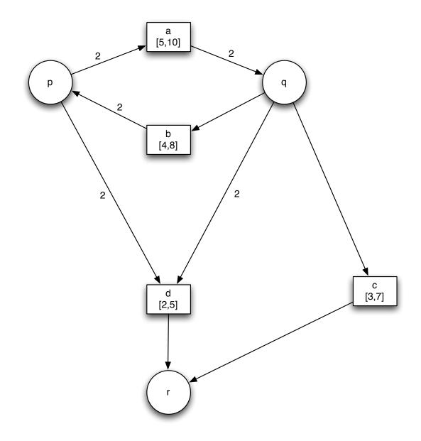
Figure 3: The transition-TPN example from Appendix C. A label on an arc indicates the arc's *weight*. For example, the arc from p to a has weight 2. This means that transition a consumes 2 tokens from place p. Arcs of weight 1 are not labelled. The interval on a transition constrains when the transition may fire, as described in Section 2.4.1.
