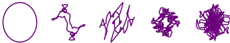
Figure 5.2: Figure showing a trajectory increasing with the depth of a network. Starting with a circular trajectory (left most pane), it is fed through a fully connected \tanh network with width 100. Pane second from left shows the image of the circular trajectory (projected down to two dimensions) after being transformed by the first hidden layer. Subsequent panes show the trajectory after being transformed by multiple layers. This figure is retrieved from Raghu et al. [6].
