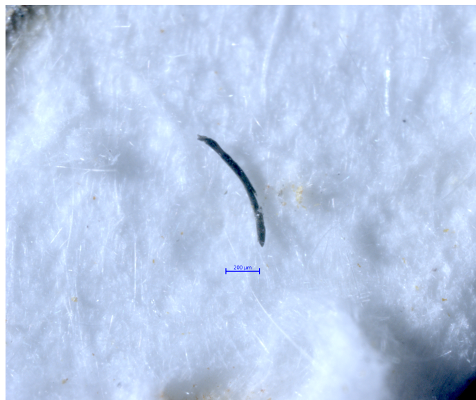
Figure C.2: Example of blue fiber found in core DRA2A, here in sample A.3-4.1. ANTHROPOGENIC PIGMENT or POLYETHYLENE .
