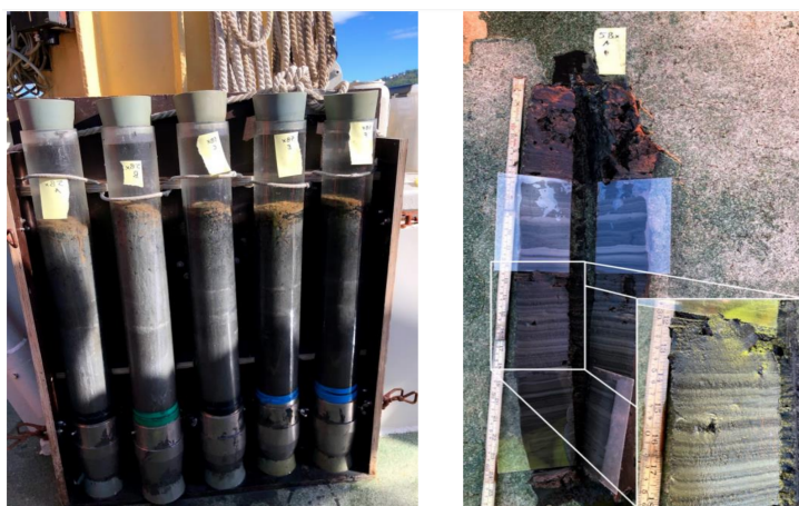
Figure 2.3: a. Sediment cores collected at station 5Bx, three deployment, six cores- one inconclusive(5BxD). b. Sediment core 5BxA pushed out on deck for sediment logging.
