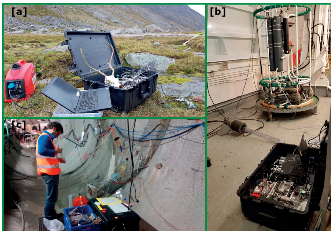
Figure 1.5: Impressions from the field work. [a] Test measurements with the miniRUEDI at the North Cape. [b] Measurements and sampling during the ‘Johan Hjort’ cruise in the North Sea. Seafloor water sampled with the CTD in the background analysed with the miniRUEDI in the front. Sediment core sampler in the center. [c] Sampling and measurements with the miniRUEDI at the rock laboratory Grimsel.
