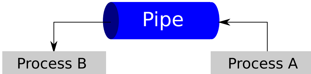
Figure 6.1: A UNIX-pipe makes it possible for two disjoint processes to share information. Data from process A is piped to process B.
