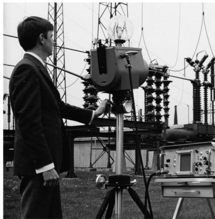
Figure 25.2 1969: Thermovision Model 661. The camera weighed approximately 25 kg (55 lb.), the oscilloscope 20 kg (44 lb.), and the tripod 15 kg (33 lb.). The operator also needed a 220 VAC generator set, and a 10 L (2.6 US gallon) jar with liquid nitrogen. To the left of the oscilloscope the Polaroid attachment (6 kg/13 lb.) can be seen.
