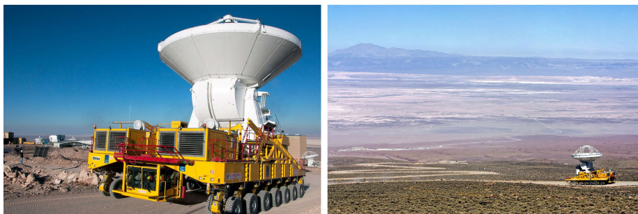
Figure 3.3: The process of moving an ALMA antenna. Seen in the photographs are the specially designed, large, high-power vehicles required to be able to move the about 100 tonnes heavy 12-m antennas at the 5 km high altitude of the ALMA site at the Chajnantor plateau. Credit: ESO/T. van Kempen (left) and AUI/NRAO, Carlos Padilla (right).
