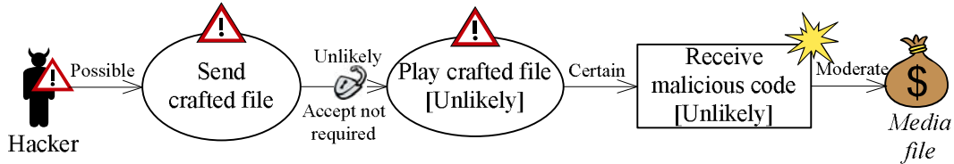
Figure 32: Example threat diagram annotated with likelihood and consequence values
