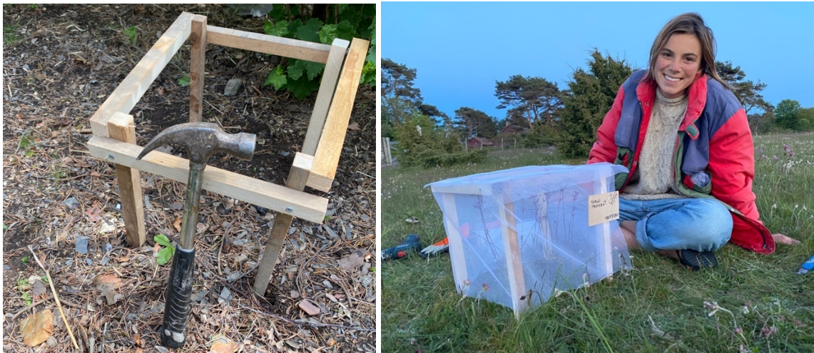
Figure B.8: The cages were built with angular legs so that they could be hammered into the ground (left). Each cage was completely covered in mosquito net (right). Photo: André Navarro.
