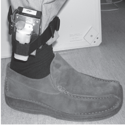
Figure 10. Motion Recording device attached to the lower leg.
