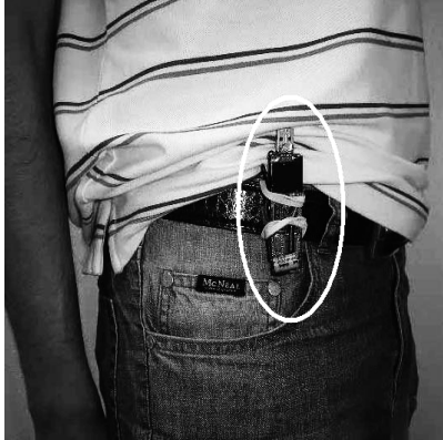
Figure 2. Pen-resembling accelerometer sensor attached to the hip [9].
