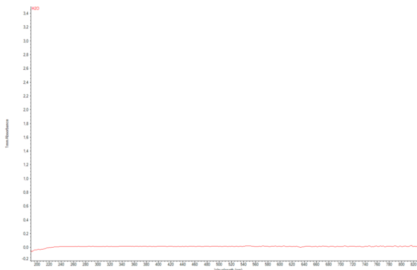
Figure 51. UV absorption spectra measured on a Nanodrop 2000 in UV-VIS mode. (1) UV-VIS spectrum for polymyxin B1. (2) UV-VIS spectrum for polymyxin E1. (3) UV-VIS spectrum of blank (Type 1 H 2 O). All samples were referenced against a blank (Type 1 H 2 O).
