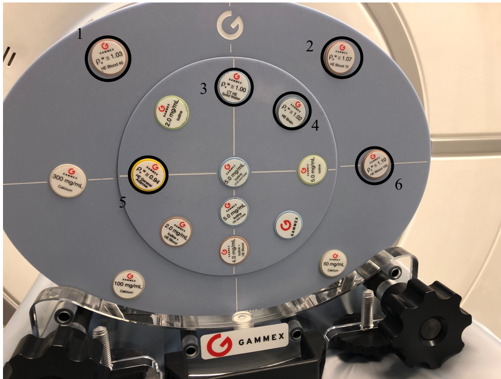
Figure 3.2: Gammex phantom where the cavities are filled with the rods. The rods that are circled around is the rods that is for HU analyses in this thesis. They are of material 1) HE Blood 40, 2) HE Blood 70, 3) CT HE Solid water, 4) HE Brain, 5) HE General Adipose, and 6) HE Blood 100. (HE: High-equivalency)
