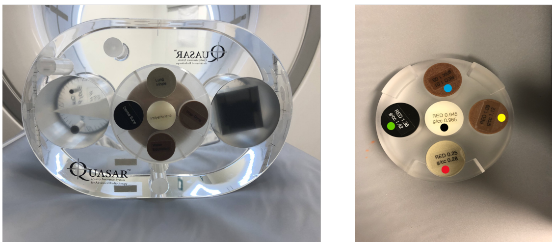
Figure 3.1: To the left the Quasar phantom with the five inserts is shown. On the left a close up image of the 5 insert are shown. The red dot shows the 'Lung Inhale', the yellow shows the 'Inner bone', the blue dot shows the 'Water Equivalent', the green dot shows the 'Dense bone', the black shows the 'Polyethylene'. In the right image the holder with the inserts is rotated 180°.
