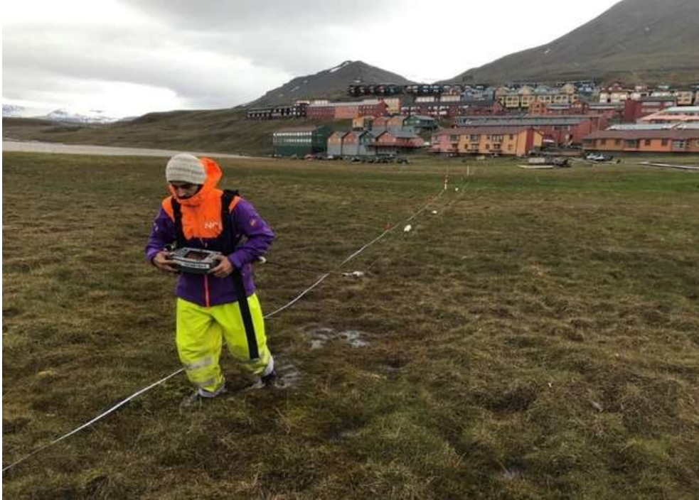
Figure 2.6: Photo of OhmMapper surveying in Svalbard. (Picture credit goes to Dr Sara Bazin).
