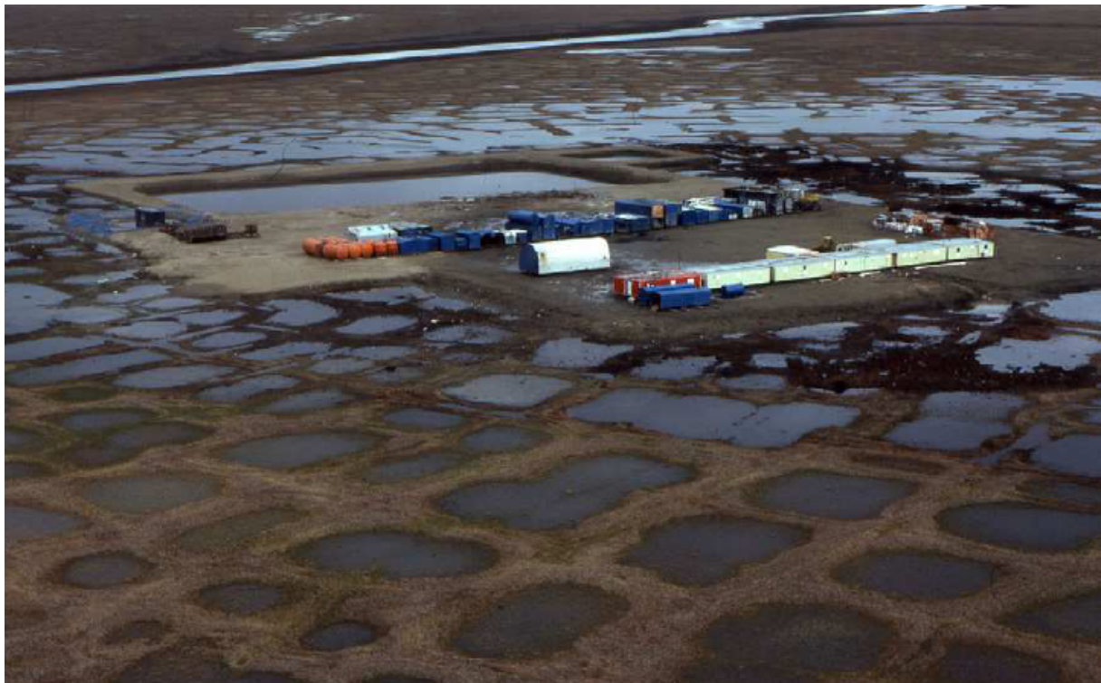
Figure 3.8: Low centered ice wedge polygons spotted in Alaskan North Slope, USA. Figure from (French, 2007).
