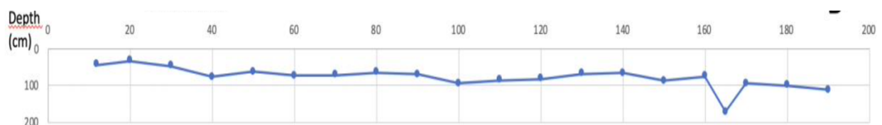
Figure 5.22: Depth of the active layer (in cm) measured in September 2017 while conducting Terrameter Survey. The average depth value is 79 cm (Bazin et al., 2021).
