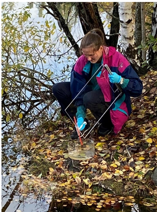
Figure 4. Sampling of the surface microlayer using the sampling plate.
