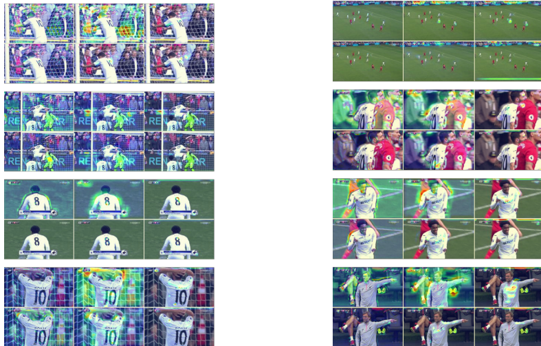
Figure 4.6: Heatmap from three of the layers of the VGG inspired model with RGB 108 \times 192 input, before and after the extra training. These background frames was previously predicted wrong.
