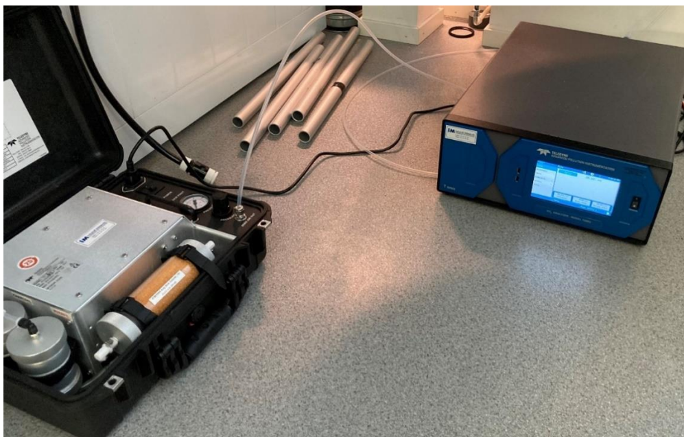
Figure 2-11: The NO 2 -analyzer (right) and its zero-air system (left) installed at OsloMet.
