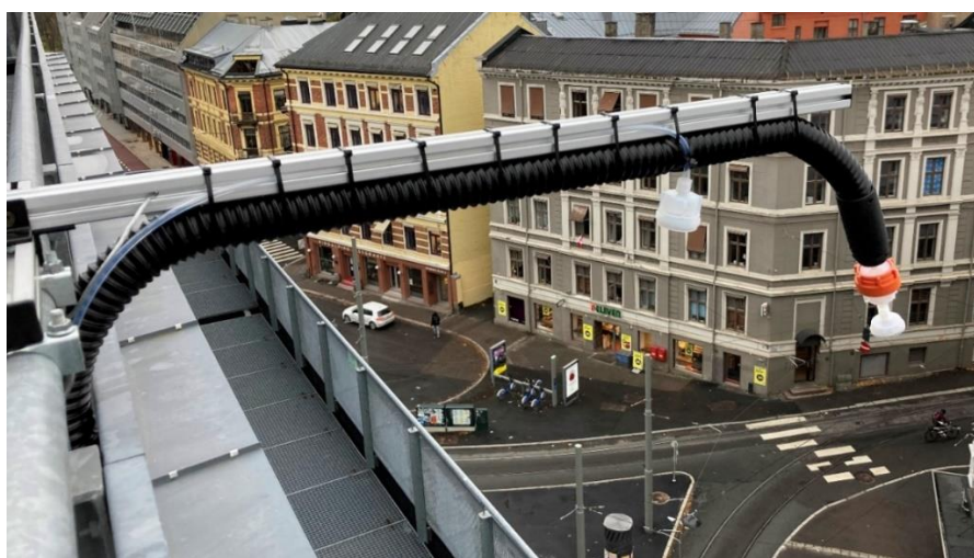
Figure 2-2 Inlet setup at OsloMet. The main inlet of the PTR-ToF-MS is heated (black covering) and equipped with both rain cap and particle filter. The clear inlet is connected to the NO 2 -analyzer and only requires the rain cap.
