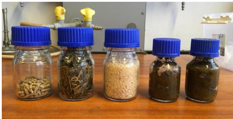
Figure 6.6: Samples collected from a cattle barn at SHF. From left: Food pellets, silage, sawdust, “old” manure, and “fresh” manure.
