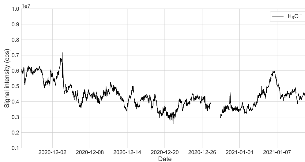
Figure 2.12: The H 3 O + -ion signal (cps) (30-second moving average) from the field measurements campaign.
