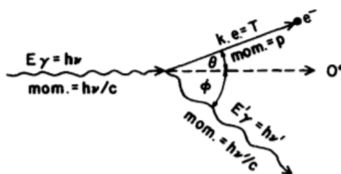
Figure 2.2: A simple sketch portraying the kinematics of the Compton effect. The wave is the photon in the interaction, the straight line is the scattered electron. \phi and \theta are the scattering angles for photon and electron respectively.[18]
