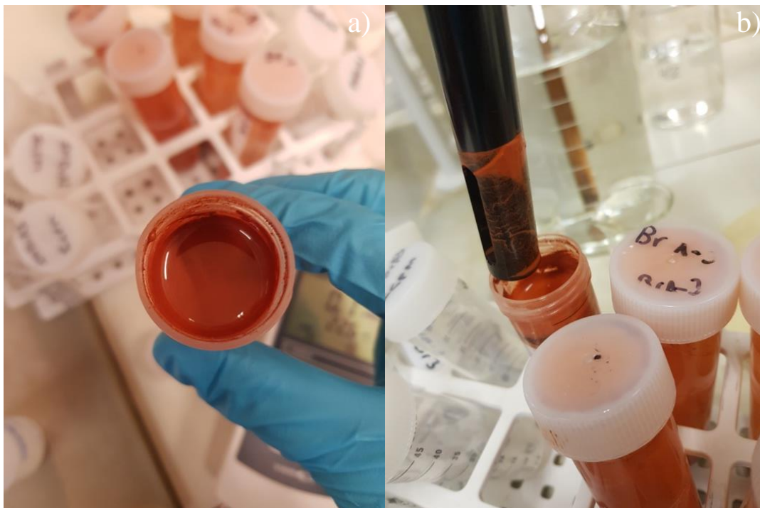
Figure 9. Picture on the left a) sample of bauxite residue with açai before measuring the EC. Picture on the right b) the electrode removing some slight amount of the solid phase.
