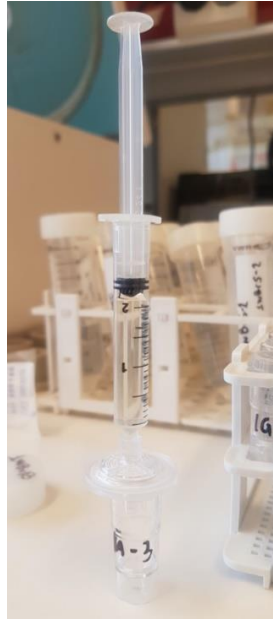
Figure 11. Sample extraction of eluent is filtered (2ml) for CFA experiment. Notice the lack of color of bauxite residue with gypsum.
