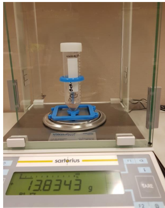
Figure 6. Measuring the weight of bauxite residue to determine the soil moisture content, taking into account the weight of the tube samples.
