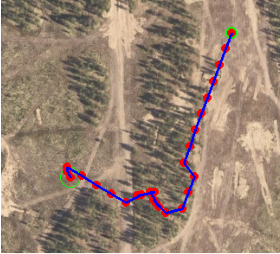
Figure 4.2: Hybrid A* with \delta = 0.25 , with additional costs for steering and velocity
