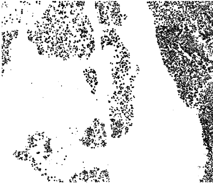
Figure 3.6: The difference between DSM and DTM from the same image as in Figure 3.4 . In addition, a threshold of 3 meters is used to remove noise.
