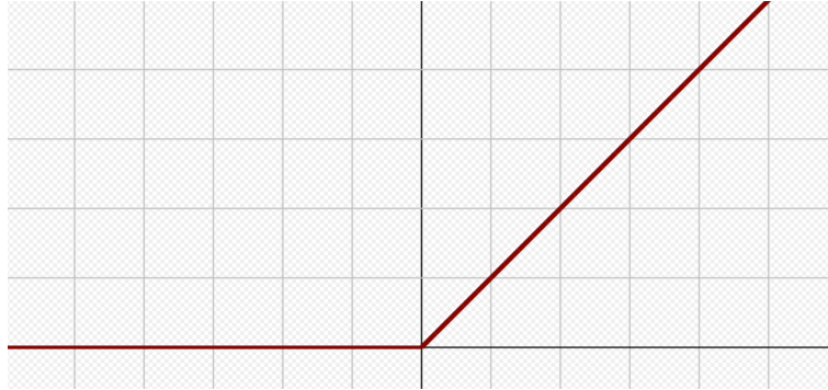
Figure 2.6: ReLU activation function. All negative values are zero and the same output as input if elsewhere. ReLU is not differentiable at zero, therefore, thresholding to zero is performed if x = 0 . Image grabbed from [15].
