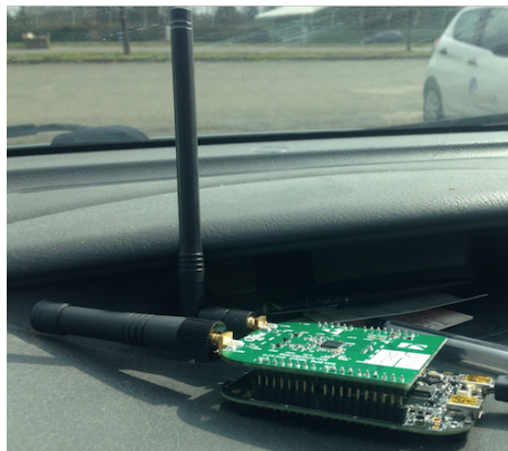
(c) Freescale KRDM-KL25Z development board with mounted SX1276 Mbed shield (credit: (Augustin et al. 2016))
