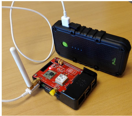
(a) Raspberry Pi with Dragino LoRa/GPS HAT (credit: (Johnsen, Bloebaum, Jansen et al. 2019))
