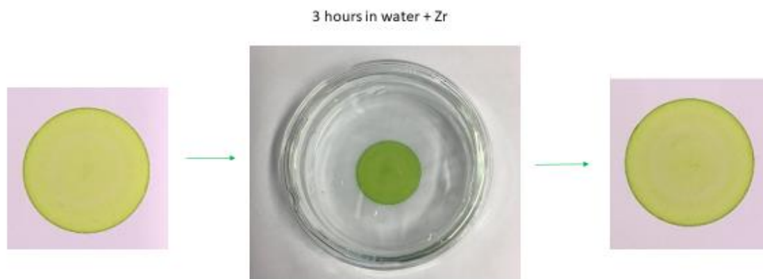
Figure 5.25: 5 layers of ZrTCPP in water with the addition of Zr do not change color.
