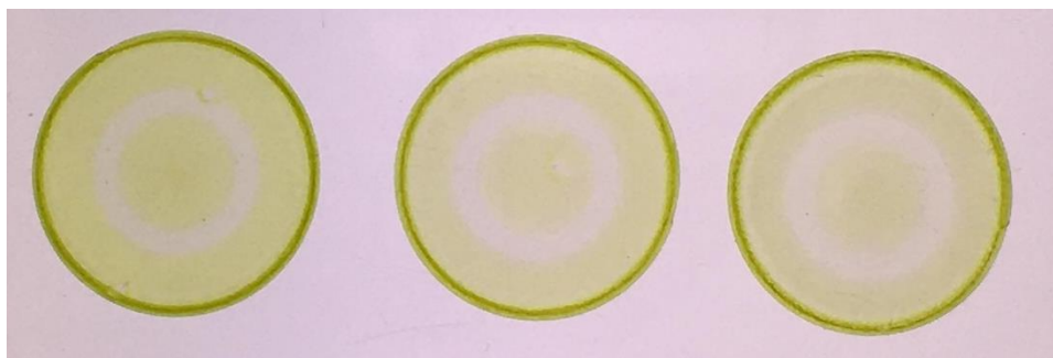
Figure 5.15. The deposition of the thin film included a washing step with ethanol. (a) 1 x EtOH. (b) 2 x EtOH. (c) 3 x EtOH.
