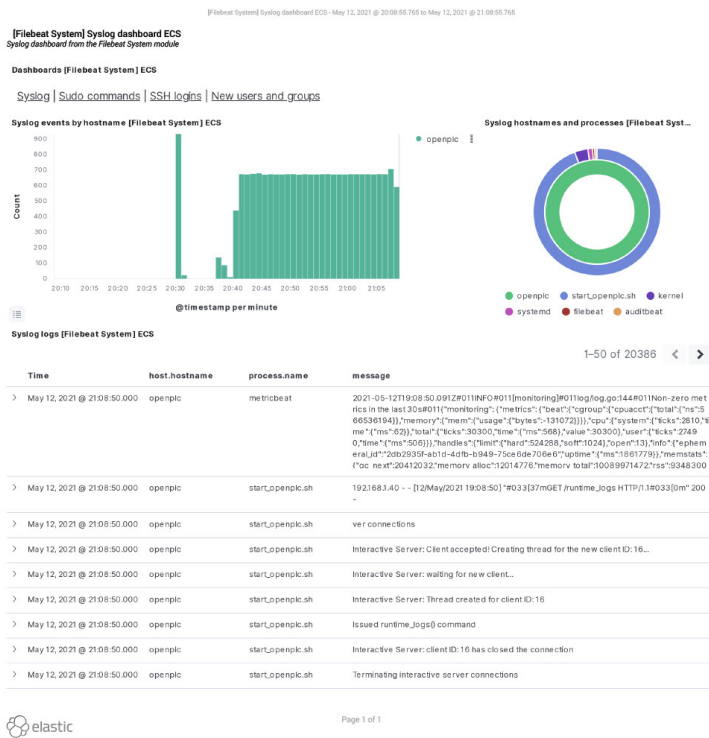
Figure 8: Screenshot with example data collected by Filebeat form the OpenPLC device shortly after starting up.
