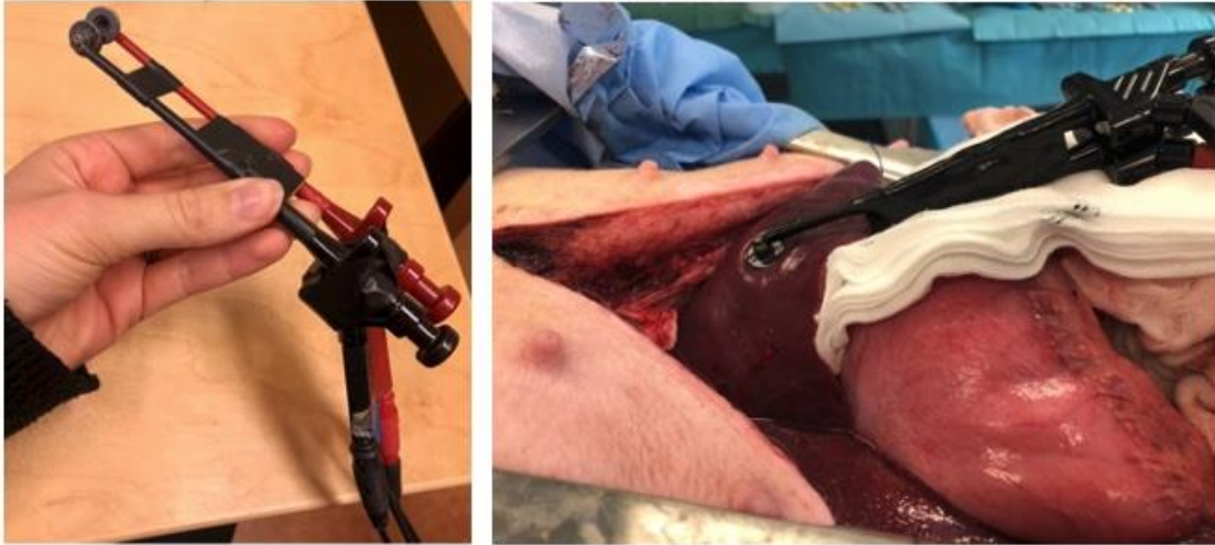
Figure 3.6: Left: two-electrode system with Ag/AgCl electrodes. Right: in-vivo measurements on liver lobe using Ag/AgCl electrodes.
