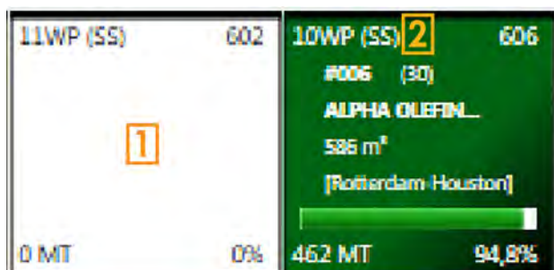
Figure 31. Single tanks in the tank plan. User interface screen elements showing a vacant tank and an occupied tank in the tank plan.
