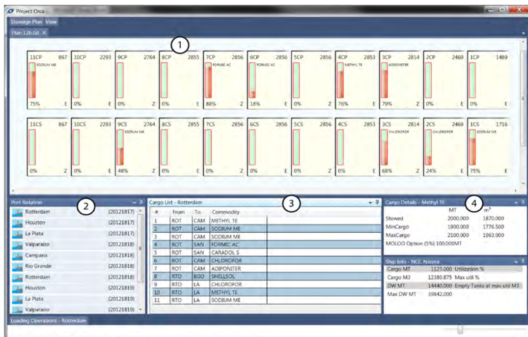
Figure 13. The first iteration of the tank plan in ORCA showing the main screen elements in the user interface: the main tank plan (1), the rotation list (2), the cargo list (3), and cargo detail/ship info (4).
