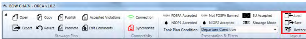
Figure 39. Operators can configure and save their own custom screen layouts by clicking on 'Save' in the Layout section of the top menu. The standard, 'factory settings' can be restored by clicking on 'Restore' in the Layout section of the top menu.
