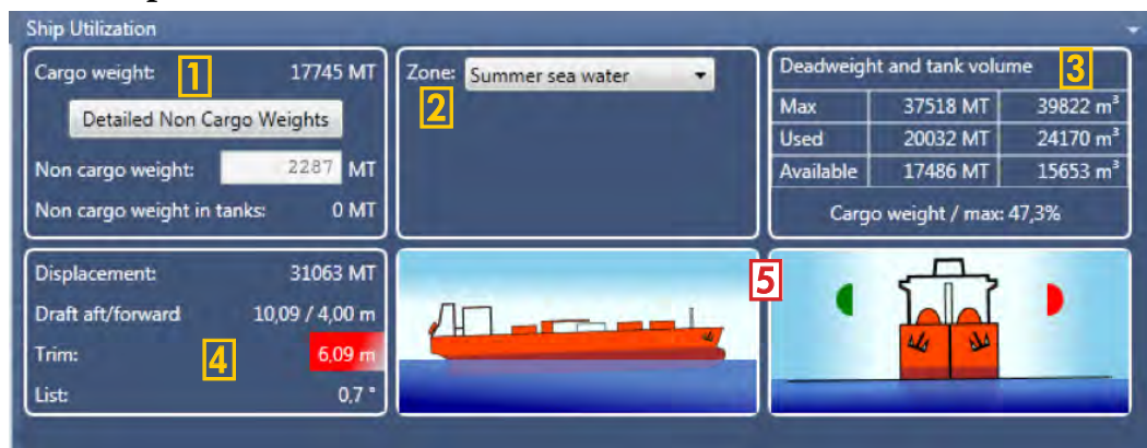
Figure 51. The Ship Utilization window visualise the degree of utilisation of the ship for the currently selected call. (Numbers in the figure correspond with the numbers in the following paragraph.)
