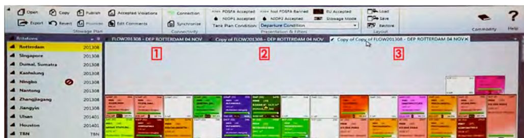
Figure 25. Duplicate stowage plans. The operator can make as many duplicates as needed. Here, the operator can try out three different stowage plans: the initial plan [1], that the operator preserved by making a copy [2], which could be used to explore other stowage constellations. This copy was, in turn, preserved by making yet another copy [3], providing the operator with an extended number of possibilities to mediate the internalisation process.
