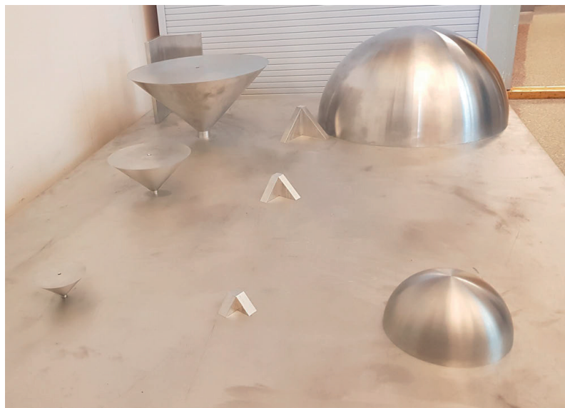
Figure 2.2: My realization of the suggested calibration target, produced by FFI's Prototype Workshop. Photo: Stig A. V. Synnes.
