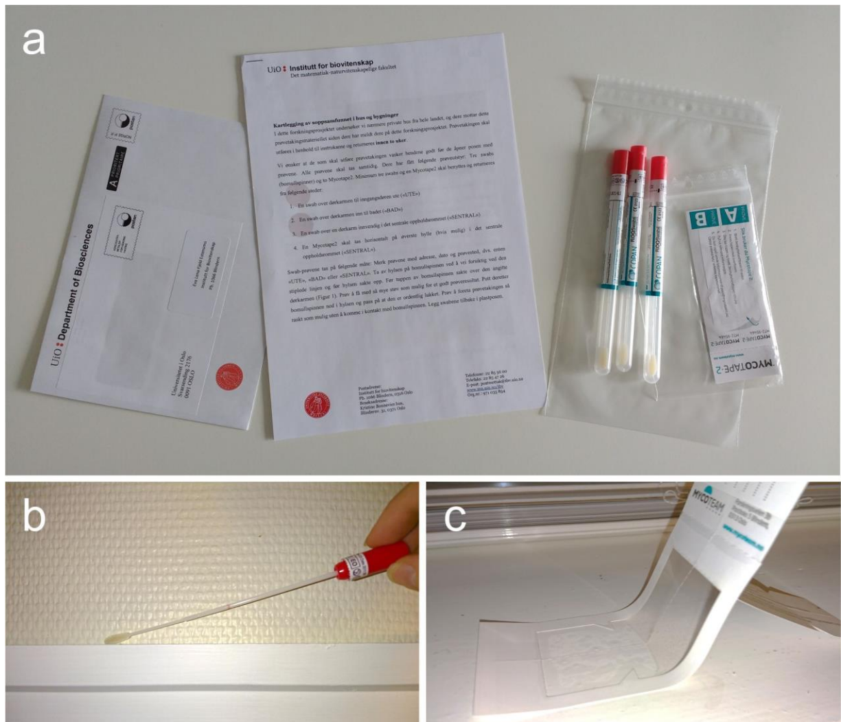
Figure S1. (a) Sampling kit sent to the volunteers, including return envelope, instructions, three FLOQSwabs (b) and two adhesive tapes (c; Mycotape2).
