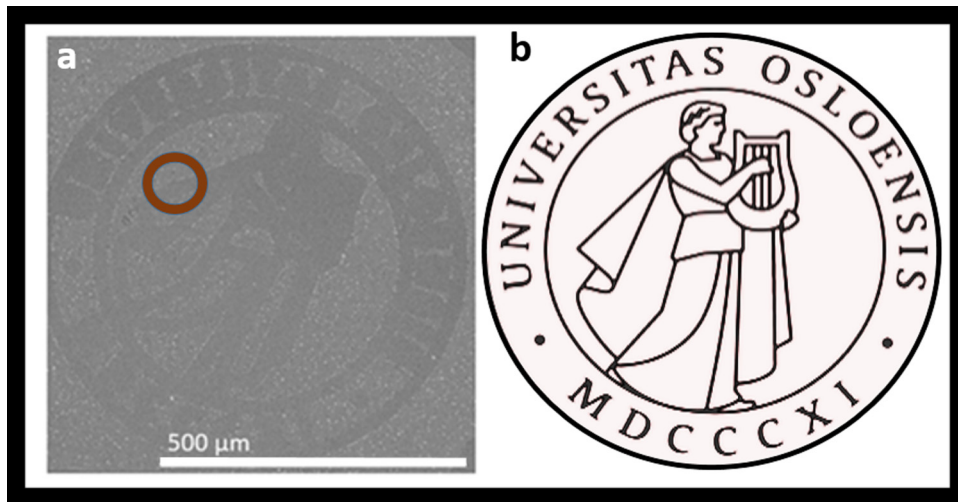
FIG. 9. SEM micrograph (a, left) illustrating the selectivity of the MoO x system as deposited on LiF. The pattern is the University of Oslo's logo (b, right). The LiF film under the lines of the logo shown in (b) was removed with lithography prior to deposition of MoO x . The circle in the micrograph is the area where the EDS measurements in Fig. 10 are taken.
