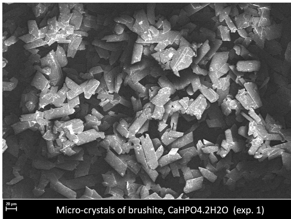
Figure S7: FESEM image showing elongated micro-crystals of brushite (size > 20 \mu m) obtained in experiment 1 (Table 1).
