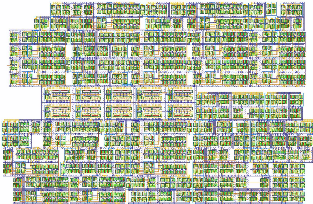
Figure 4.35: Layout of the top layer. 93.98\ \mu\text{m} x 60.75\ \mu\text{m}
