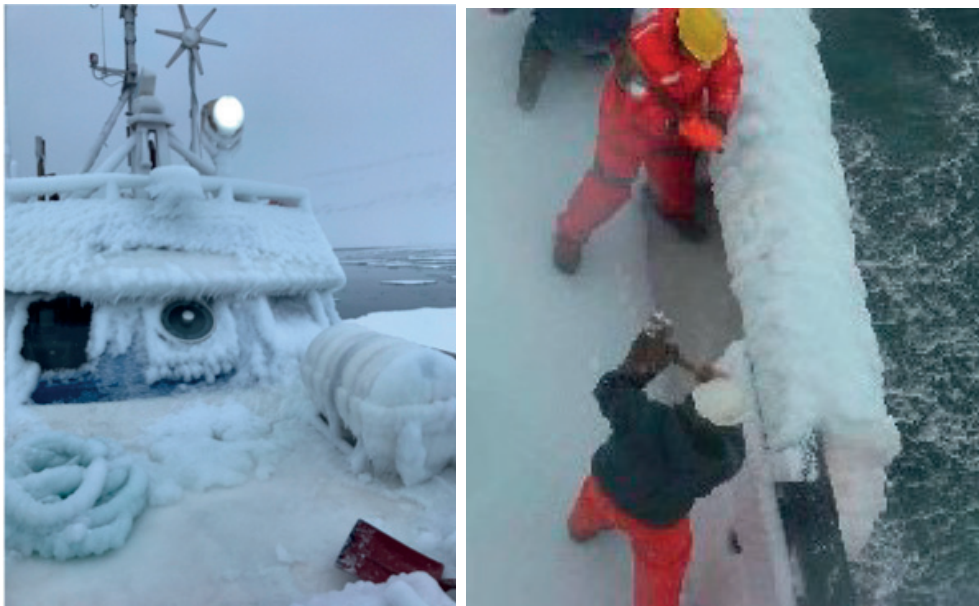
Figure 1.1: Marine Icing examples. To the left, photography from field measurements in Svalbard (Picture taken by Atle Jensen, 2017). To the right, crew of ship removing icing obtained from Cook and Chatterton 2008.
