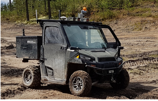
Fig. 4. Olav, the autonomous UGV used in the experiment.
