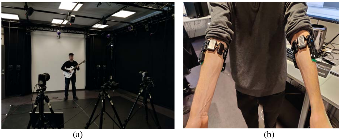
Figure 2. (a) A participant during the recording session. Motion capture cameras are visible hanging in the ceiling rig behind and on stands in front of the performer. The monitor with instructions for the performer can be seen below the front left motion capture camera. (b) The protocol used for placement of the EMG electrodes: Two Delsys EMG sensors were placed on each side of the arm corresponding to the extensor carpi radialis longus and flexor carpi radialis muscles, just below the Myo armbands.
