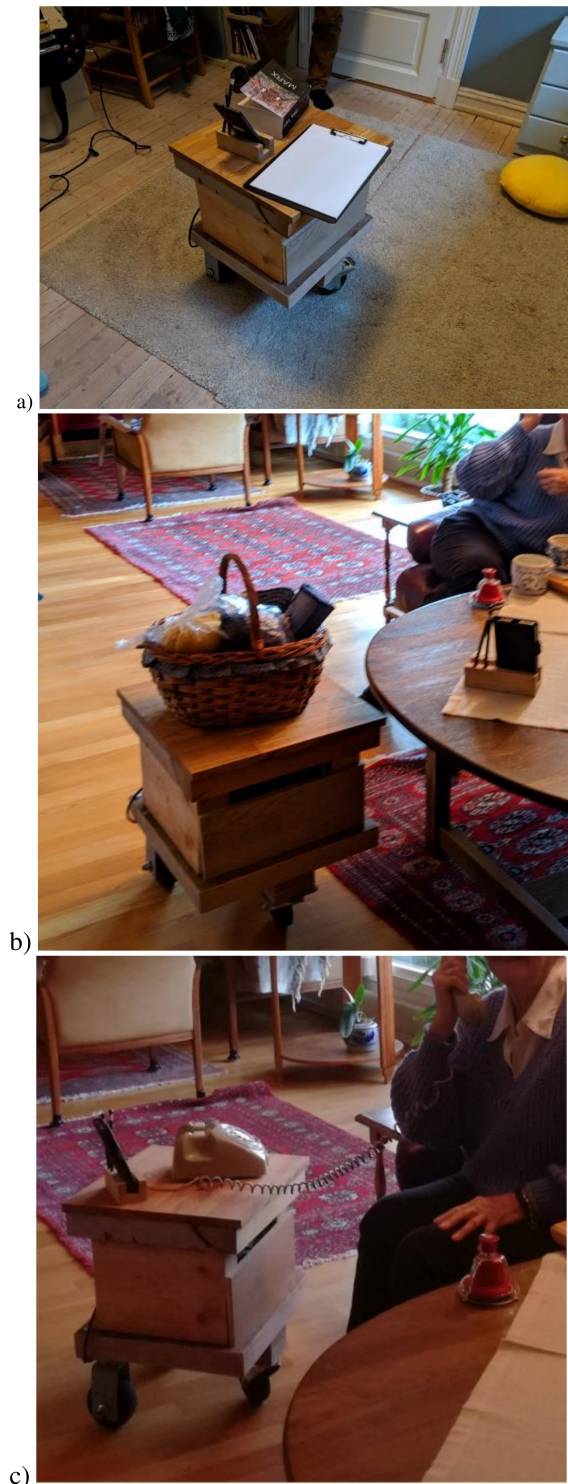
Figure 4. a) and b) Prototype of T-ABLE transporting things in the home c) Prototype of T-ABLE where an elderly participant uses it to bring the home fixed phone and the mobile phone closer to her
